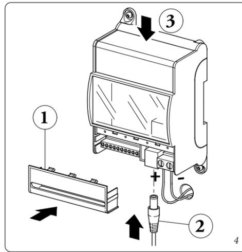
After the boiler and the Wi-Fi module have been powered (Fig. 4, Ref.2) wait about 30 seconds before configuration in a way that the communication between Wi-Fi module and boiler has established.
