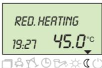
Permanent functioning of heating and d.h.w. modes according to the reduced temperatures setting (see pages 6 and 24).
