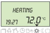
Permanent functioning of heating and d. h. w. modes according to temperatures settings (see page 6).
