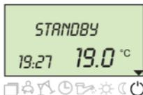
Turn off of the system with anti freeze protection on (heating and d. h. w. modes deactivated).
