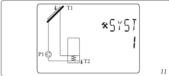
Tank 1 charging is possible if the temperature difference “dt” between the collector (T1) and tank 1 (T2) is sufficient.
