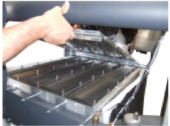
- Lift the rear burner block slightly and take out 2 pins with a 5 mm hex key, until you reach holes "C" (left and right side).
