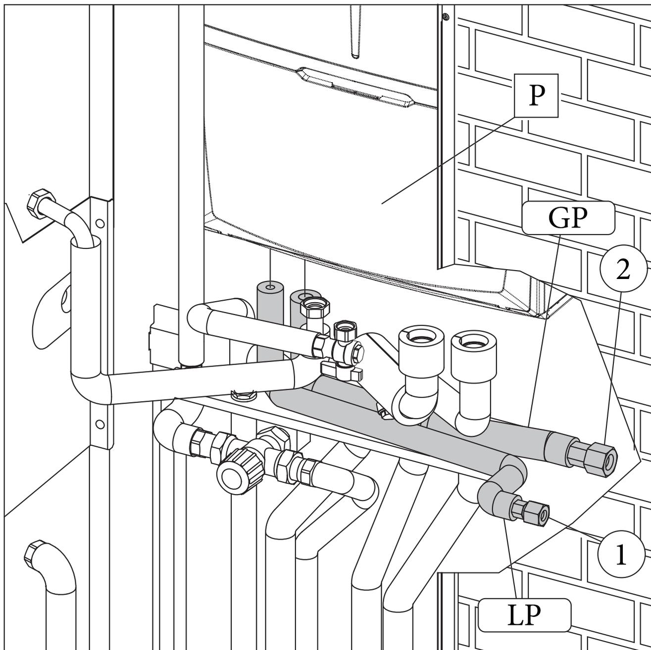
Using the pipes inside the accessories box, make the remaining hydraulic connections between the Storage Tank Unit (a), the Single-zone hydraulic unit (c) and the Magis Pro V2 Indoor Unit (P), as shown in Fig. 17.
