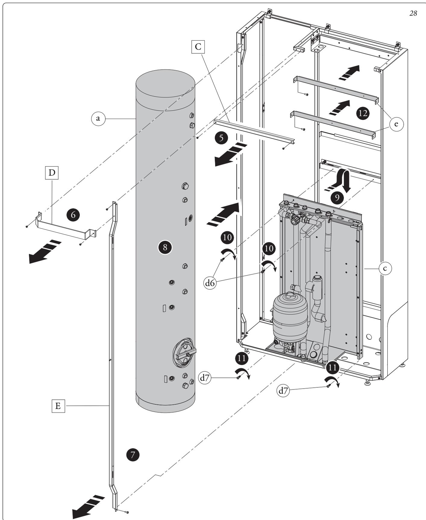
Assemble the storage tank emptying tap with its connection pipe identified with the initials AF (fig. 29). Connect the storage tank unit (a) with the single-zone hydronic group (c) with the previously assembled group.
