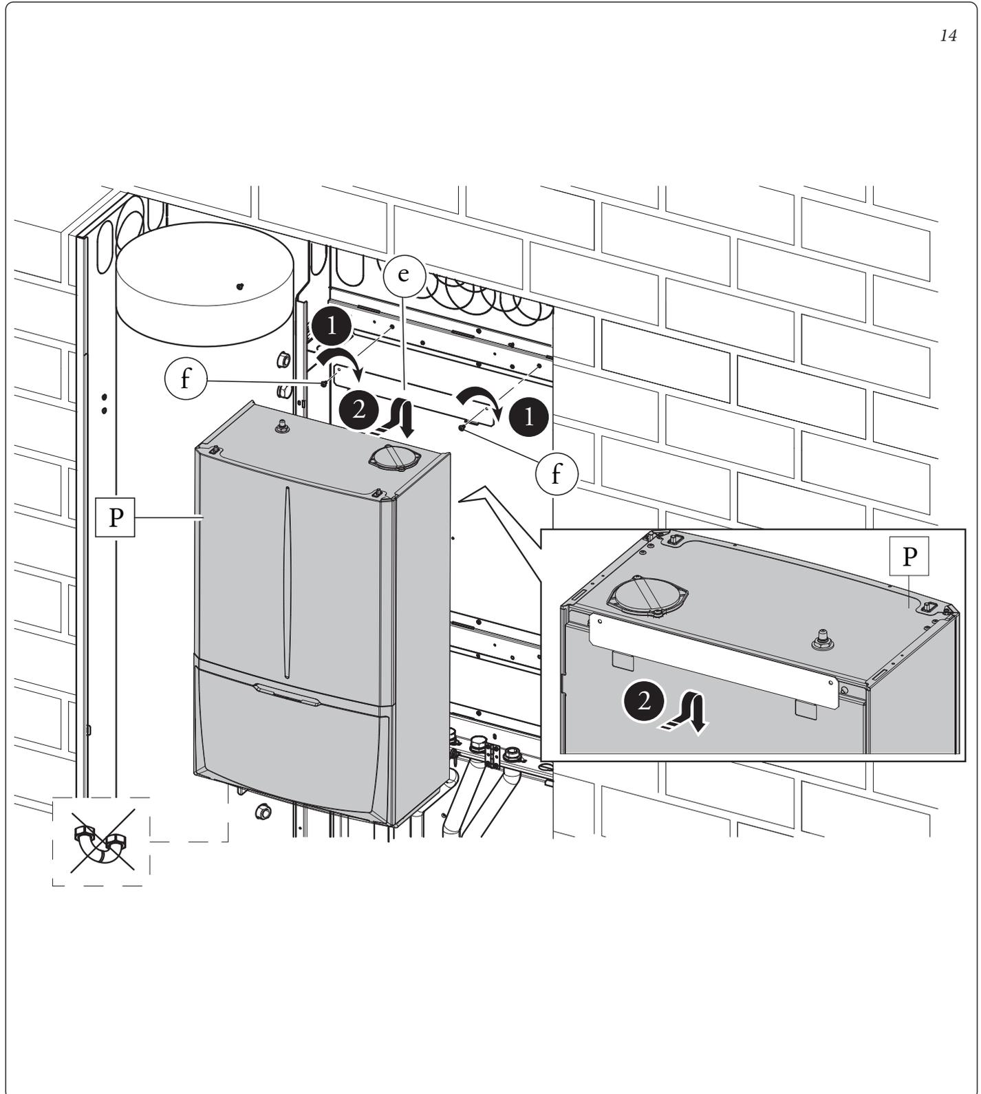
**Attention:** (Fig. 15) Remove the grill and the square gas tap from the Magis Pro V2 Indoor Unit. Remove the square tap positioned on the return of the Magis Pro V2 indoor unit and insert the Y filter with the relative connection pipes as shown in Fig. 15.
