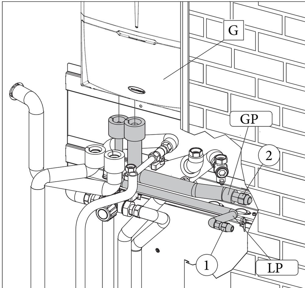
Using the pipes present inside the accessories box, make the remaining hydraulic connections between the boiler unit (a), the single-zone hydraulic unit (c) and the Magis Combo Plus V2 indoor unit (G), as shown in Fig. 22.
