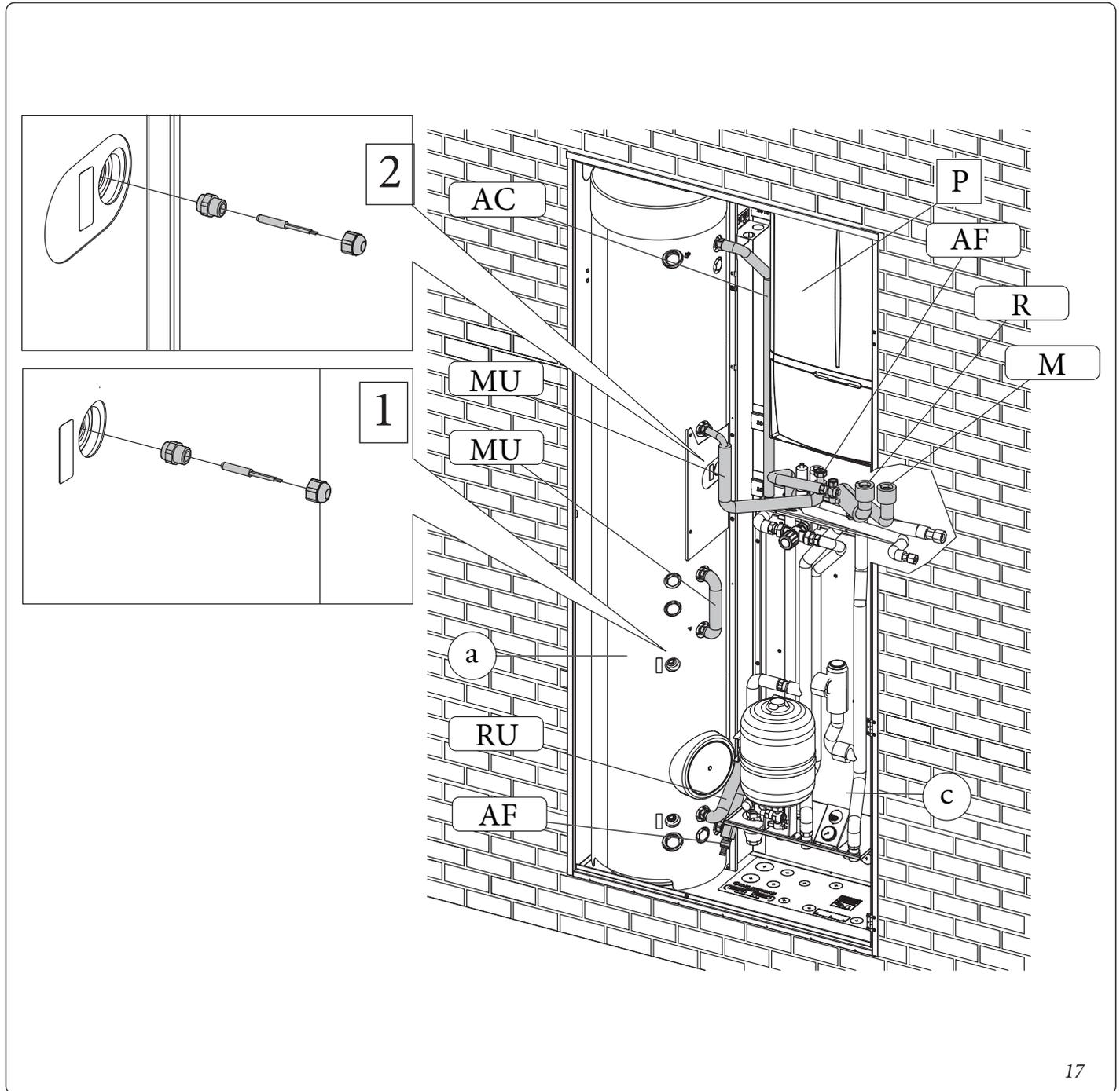
**Magis Combo Plus V2 Indoor Unit installation operations in Solar Container.**
