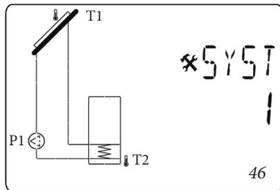
Tank 1 can be loaded if the temperature difference “dt” between manifold (T1) and tank 1 (T2) is sufficient.
