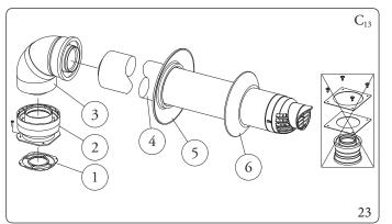
The adapter kit includes (Fig. 23): N°1 Gasket(1) N°1 Adapter Ø 80/125 (2)
