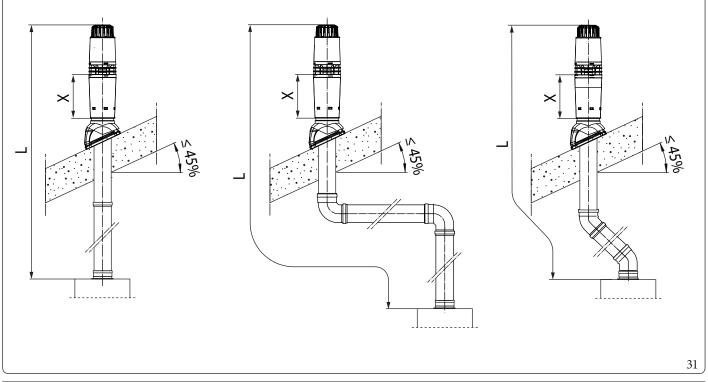
To calculate the equivalent length of the flue (L), simply add, for each component you intend to use, the corresponding value indicated in the column "Length equivalent to m of pipe" in the table in par. 1.15, and check that the resulting sum is equal to or less than the maximum length (L max) indicated in par. 1.16. ( $L \le L$  max).
