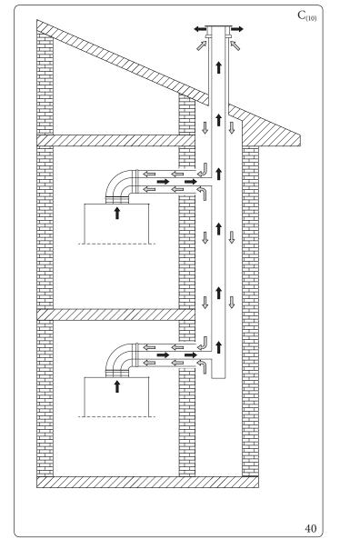
Installation in  $C_{(10)}$  configuration of an Immergas appliance (only permitted with approved original flue, including the specific non-return valve), makes it possible to intake combustion air directly from the shaft where the flue gas exhaust is present in the collective flue.
