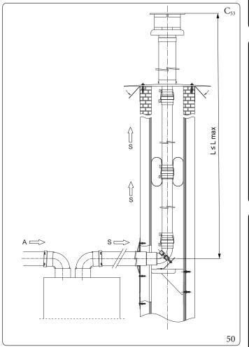
The maximum lengths ((Lmax) of the various flues that can be installed are given in the summary table in parag. 1.16.
