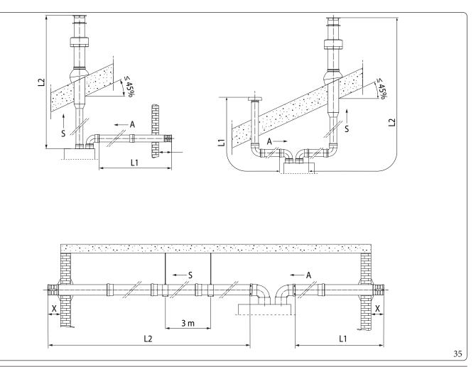
To calculate the equivalent length of the flue (L), simply add, for each component you intend to use, the corresponding value indicated in the column "Length equivalent to m of pipe" in the table in par. 1.15, and check that the resulting sum is equal to or less than the maximum length (L max) indicated in par. 1.16. ( $L \le L$  max).
