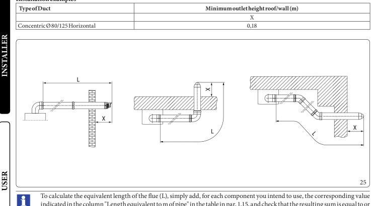
To calculate the equivalent length of the flue (L), simply add, for each component you intend to use, the corresponding value indicated in the column "Length equivalent to m of pipe" in the table in par. 1.15, and check that the resulting sum is equal to or less than the maximum length (L max) indicated in par. 1.16. (L  $\leq$  L max).
