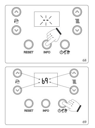
Press and hold the "INFO" button for more than 5 seconds. The display will show two dashes "--" flashing. Now enter the password ([-]) to access the programming menus.
