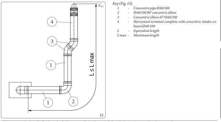
To calculate the flue length of other types of installations, follow the logic illustrated in this example.
