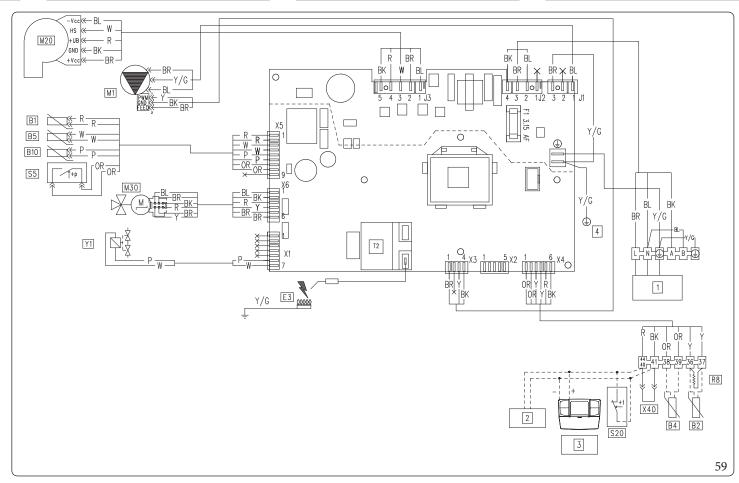
Comando Amico Remoto<sup>v2</sup>: the boiler is prepared for the application of the Comando Amico Remoto remote control<sup>v2</sup> (CAR<sup>v2</sup>), which must be connected to clamps 41 and 44/40 of the terminal board (located in the boiler control panel) respecting the polarity and eliminating link X40.
