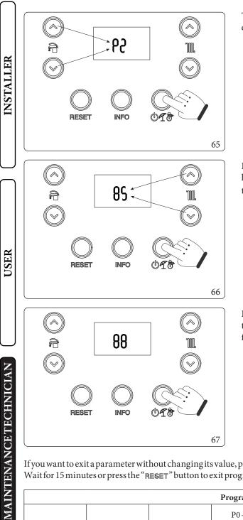
The first digit of the central indicator (Fig. 57) shows the family of the parameter, while the second digit shows its number.
