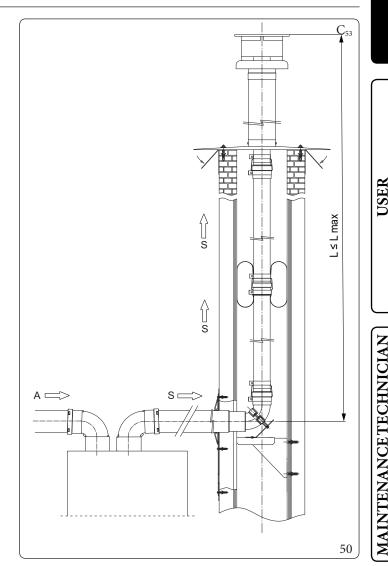
The maximum lengths ((L max) of the various flues that can be installed are given in the summary table in parag. 1.16.
