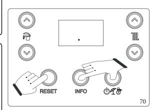
The function is activated from boiler in "off" by pressing and holding the " **RESET**", "INFO" and "**()4b**" buttons for more than 5 seconds.
