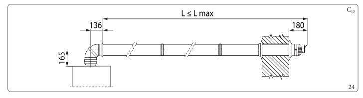
The maximum lengths ((L max) of the various flues that can be installed are given in the summary table in parag. 1.16.
