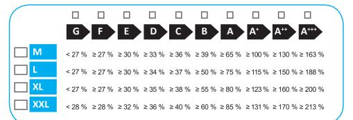
Water heating energy efficiency class in colder and hotter climate conditions
