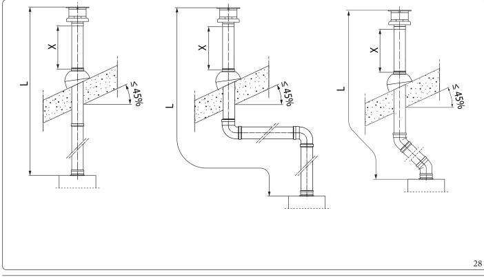
To calculate the equivalent length of the flue (L), simply add, for each component you intend to use, the corresponding value indicated in the column "Length equivalent to m of pipe" in the table in par. 1.15, and check that the resulting sum is equal to or less than the maximum length (L max) indicated in par. 1.16. ( $L \le L$  max).
