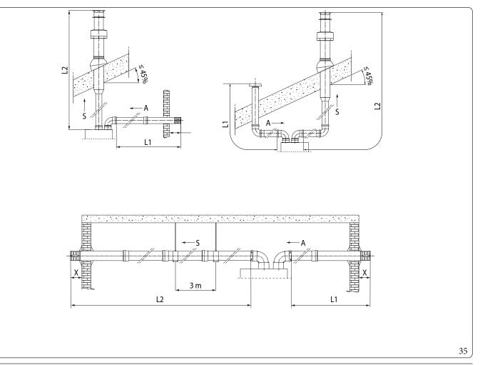
To calculate the equivalent length of the flue (L), simply add, for each component you intend to use, the corresponding value indicated in the column "Length equivalent to m of pipe" in the table in par. 1.15, and check that the resulting sum is equal to or less than the maximum length (L max) indicated in par. 1.16. ( $L \le L$  max).
