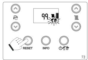
To activate the chimney sweep function, press the "**RESET**" button until activation of the function in the absence of DHW requests.
